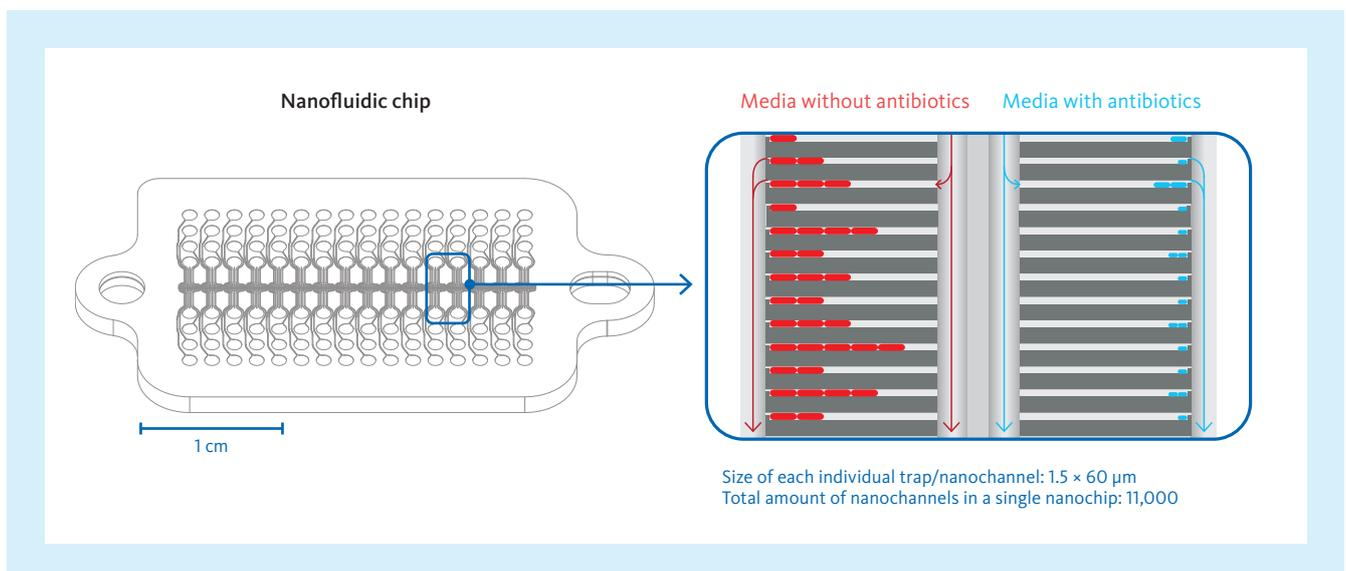
Fig. 3 Sample flow through the nanochannel system. Different conditions (represented by the different colours) are applied to each subset.
